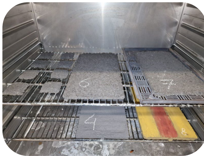
Figure 14: Stabilisation of the test specimens in an oven.
